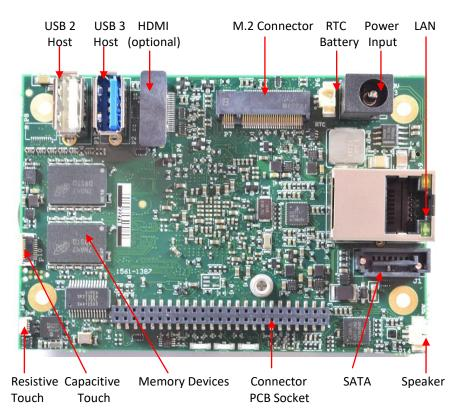
The connectors and key devices mounted on the bottom of the XE1 are:
